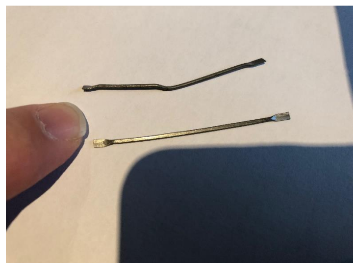
Figure 3 Steel fibres used to reinforce floor screeds and concrete
