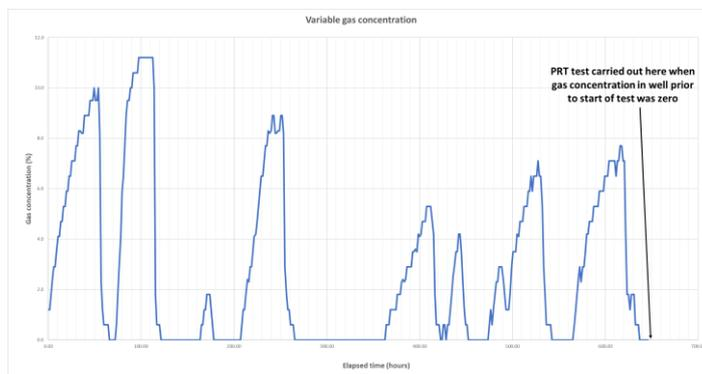
**Figure 9 PRT test carried out when there is negligible gas in the well**
