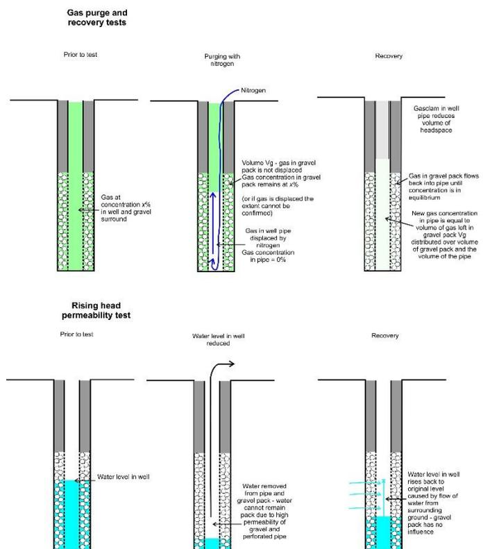
Figure 1 comparison of purge and recover test and rising head permeability test
