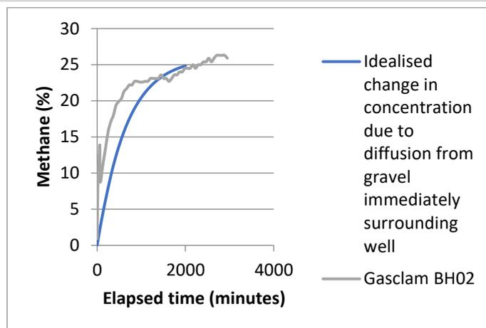
Figure 5 Analysis of gas recovery by diffusion into well from gravel pack
