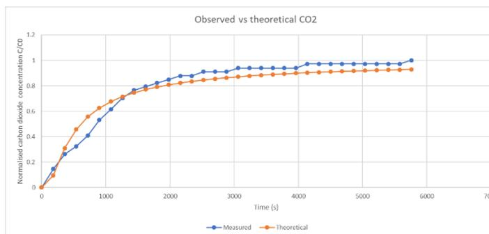
**Figure 11 Curve fit for carbon dioxide in a PRT test**
