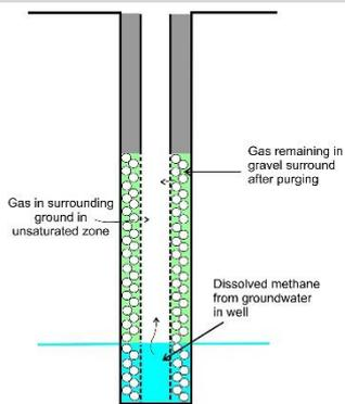
Figure 2 Sources of gas in purge and recovery test
