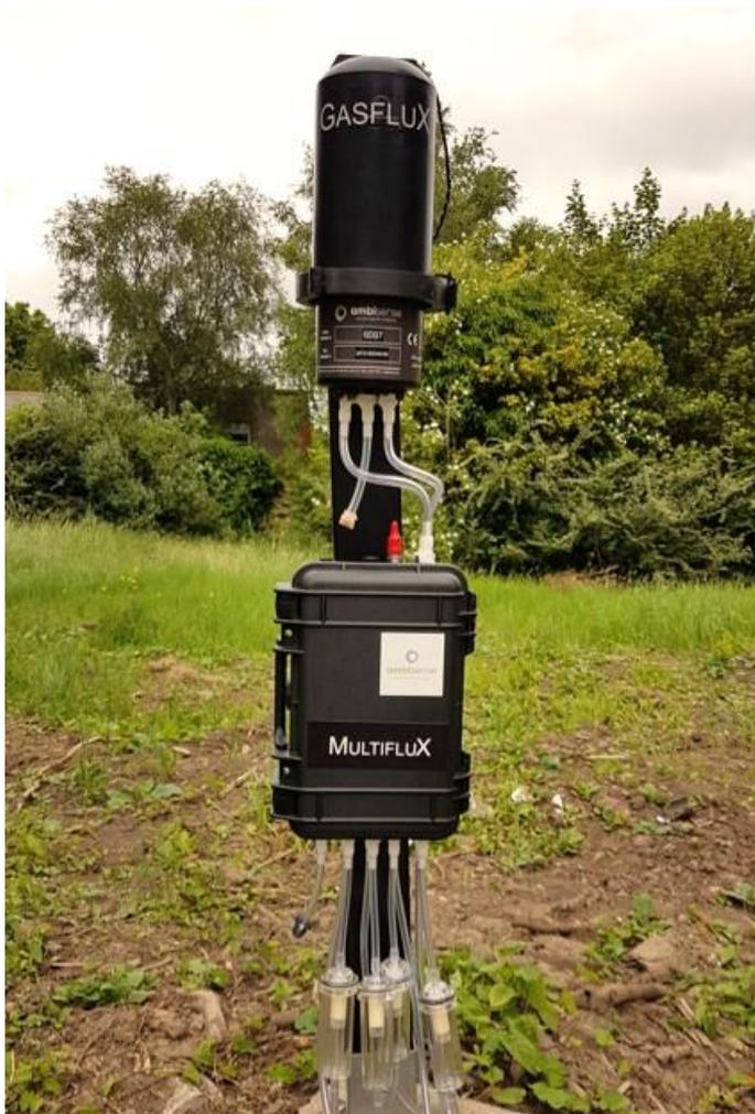
**Figure 10 Continuous monitor with manifold to take readings at different depths within a single well**
