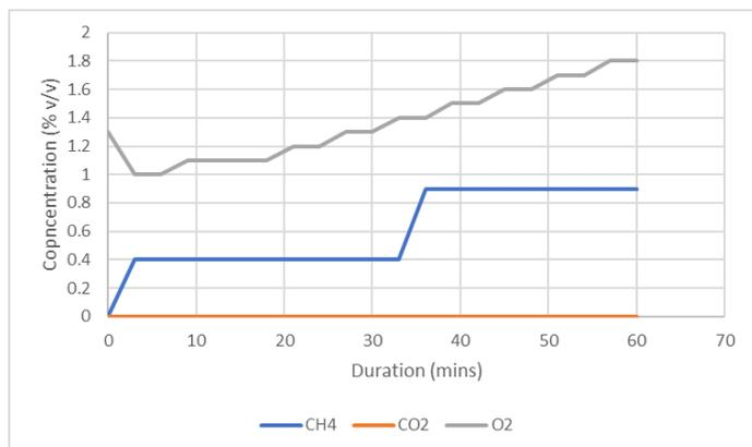
**Figure 7 Limited increase in methane concentration during PRT**
