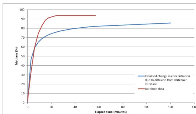
**Figure 6 Comparison of test result to predicted recharge from groundwater**
