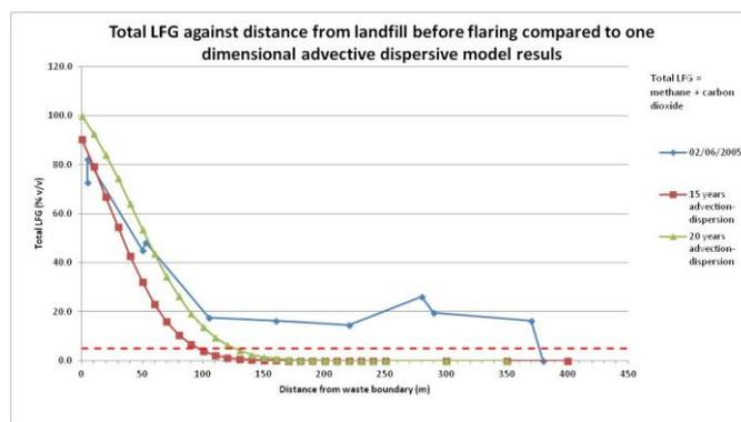
Figure 5 Comparison of model results with monitoring data
