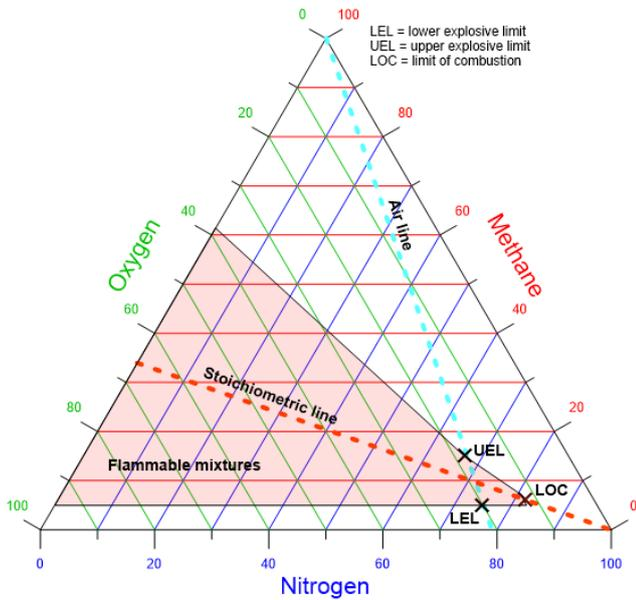
Figure 1 Flammability diagram for methane
