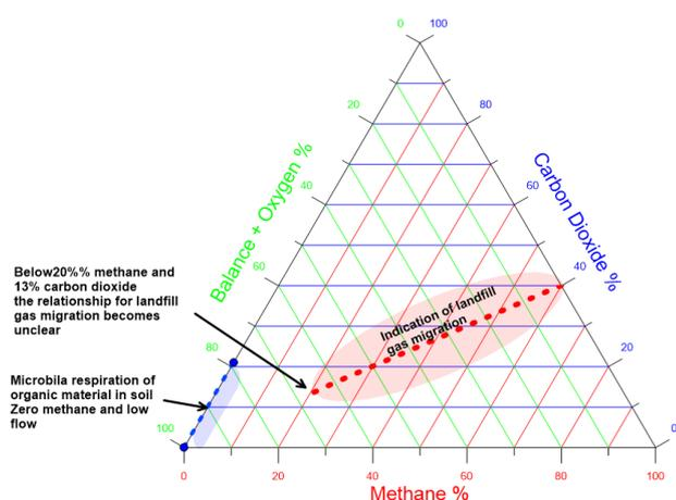
Figure 6 Ternary plot showing aerobic soil respiration zone and landfill gas migration zone
